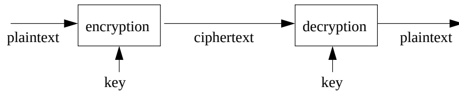
Figure 2.1: Encryption and decryption
