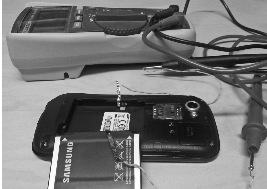
Figure 4.5 The Google Nexus S smartphone with a multimeter connected for measuring current
