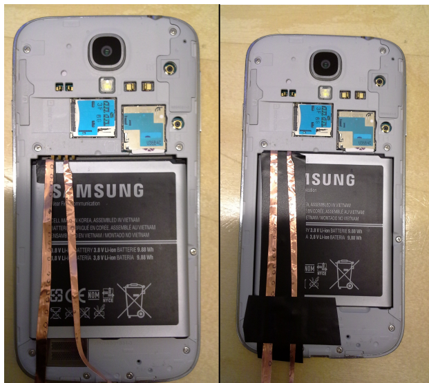
Figure 2: Voltage (+) and Ground (-) connectors bypassed with foil tape.
