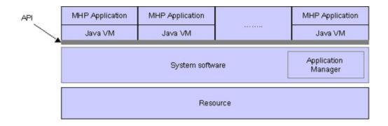
Figure 1: MHP basic architecture
