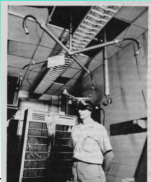
FIGURE 3--The mechanical head position sensor in use
