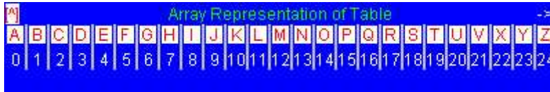
Figure 5: The hotspot in the upper left corner of an array pops up a menu. The hotspot in the upper right corner resizes the array.
